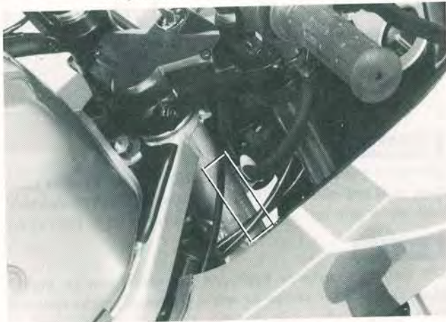
The frame serial number is stamped on the steering head's right side.
